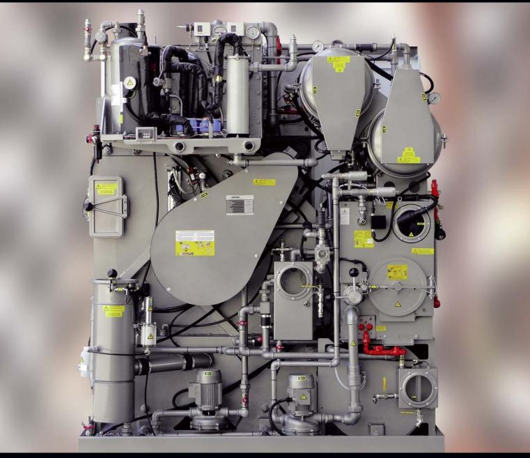
All Union models XP-XL 8000 Series are fitted with still maximum level sensors. The still level alarm is indicated in the DIALOG computer display. To ensure adequate maintenance of the still, all models are available with the automatic cleaning system STILLMATIC.
