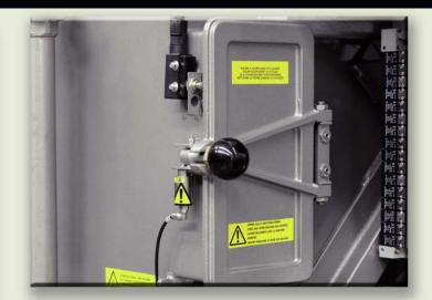
The new recovery circuit equipped with a high power ventilation system will drastically reduce drying time compared to models currently in the market. For total protection of the refrigeration unit all models of the **XL** and **XP 8000** Series are fitted with a double air filter which is easy to inspect and clean through access to one convenient panel.
