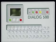
New UNION innovations for a "winning plus" ideal. The integrated control system DIALOG represents the interface proposed by UNION to optimise performance of our drycleaning machines. The large bright screen of the DIALOG computer displays all information regarding the functions of the programme and the condition of the machine components. The DIALOG computer is equipped with the useful "Programmed maintenance" facility which reminds the operator to carry out the very
